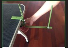
Place the C-clamp over the edge of a suitable table or work bench and rotate the thumb knob until the clamp is tightly secured to the table. Adjust the desired height of the L-shaped bracket by loosening the 2 screws and sliding the bracket vertically. Then retighten the screws.
